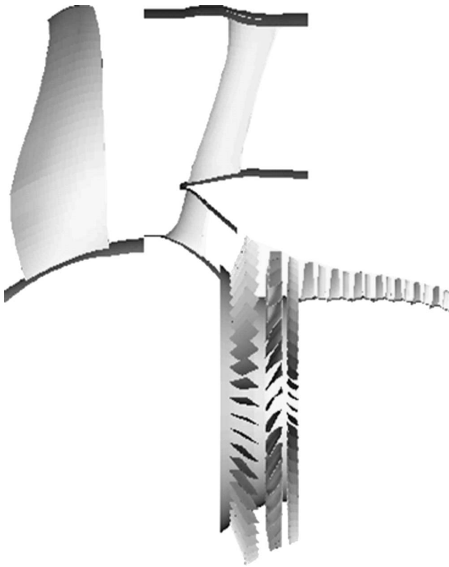
Fig. 4 Hybrid single-passage, whole-annulus model
