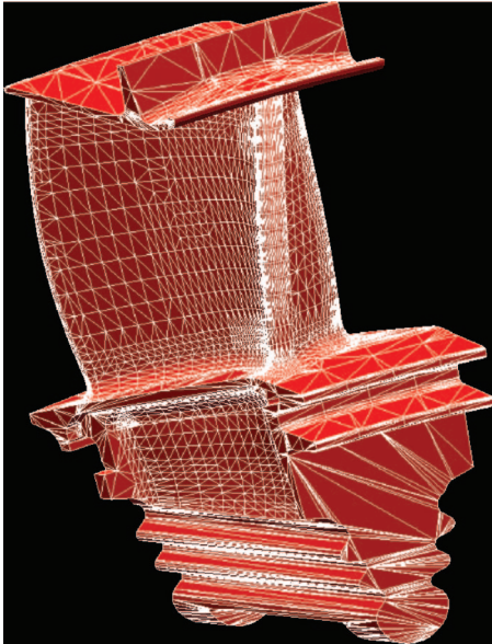
Fig. 1 Typical tessellated surface extracted by CAPRI (Haimes and Follen [10]) from a Parasolid solid model of a turbine
