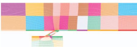
Fig. 8 Computational grid for baseline round hole case
